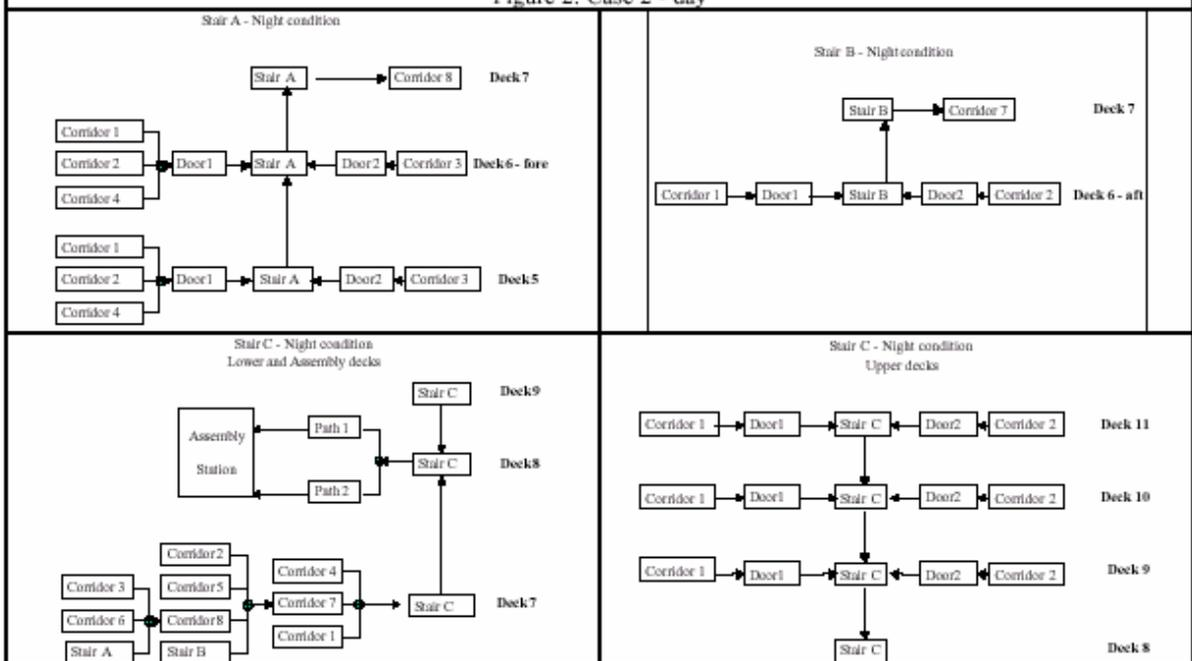
Figure 3: Case 1 (night) – hydraulic network schematisation
